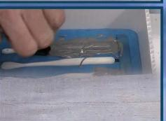
**Cast:** Slowly pour the resin in to one corner of the mold which allows the resin flow around the master reducing the risk of air entrapment.
