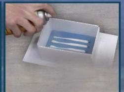
**Mold Box:** Build a mold box around the clay, seal with hotmelt glue, and spray originals and clay with Alumilite's UMR release agent.
