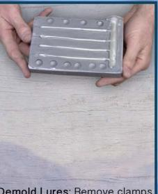
**Demold Lures**: Remove clamps and separate the mold.
