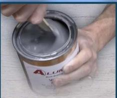
Mix each side of VAC 50: Using separate stir sticks, stir each side and re-suspend any aluminum powder that may have settled to the bottom.
