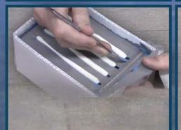
**Clean-Up:** Remove all clay away from the originals. Any clay left behind and against the original may cause excessive flash and clean up on the lures.
