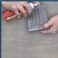
Mold Release: Prior to injecting your first parts, spray a light coat of UMR release.
