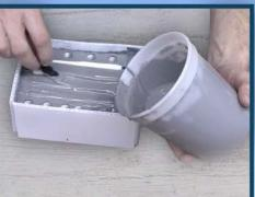
Cast: If you have a highly detailed master, brush initial coat over originals and backfill with remaining resin.
