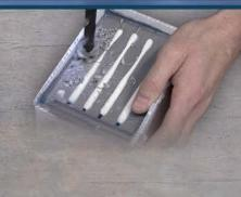
Locators: Drill shallow ¼" locator holes around perimeter of mold. These will allow the two halves of the mold to align properly.
