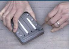
Remove originals: Remove clay originals from mold halves while being careful not to scratch or damage the mold sufaces.
