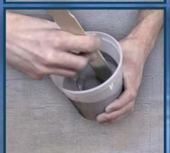
Mix VAC 50: Combine into a mixing cup and stir thoroughly ensuring to scrape the sides and bottom.
