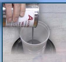
Measure VAC 50: Using a scale, measure out equal amounts of side A and B by wtt.
