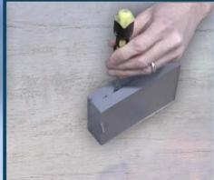
Demold: Once cured scrape away any overlapping resin and identify parting line. Gently pry apart.
