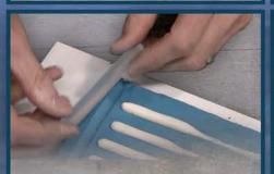
Injection Ports: Next channel in your sprew and injection ports. Again, embed them into the clay half way. We used a section of hot melt glue stick for the main injection channel.
